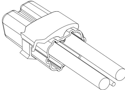
7. TO REMOVE, INSERT SCREWDRIVER BETWEEN THE CLOSING TABS AND TWIST TO OPEN THE CLAMP. REMOVE CAP SLOWLY FROM CONNECTION ALLOWING GEL TO REMAIN IN CAP.
