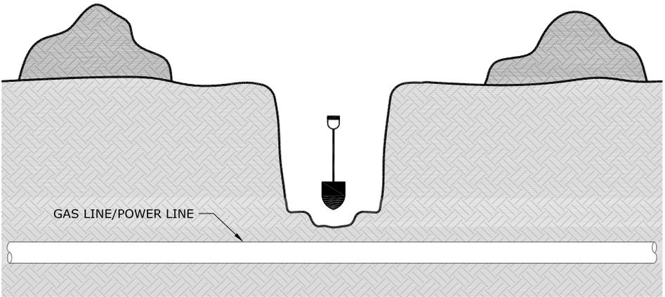
Dig a trench by hand across the full width of the excavation (perpendicular to or "across from" the line). If the line is not uncovered, mechanically excavate to one half the depth of the trench. Repeat this process until the line is exposed.
