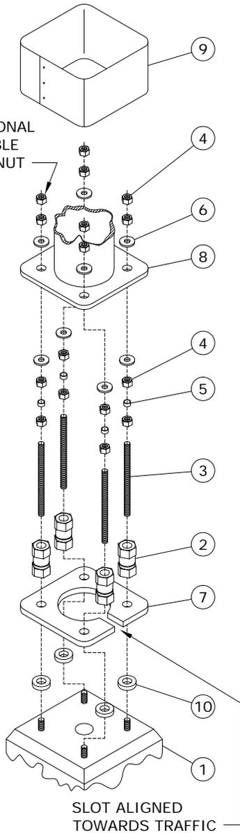
1. CLEAN THE TOP SURFACE OF THE CONCRETE BASE AND ENSURE SURFACE IS FLAT AND LEVEL WITH NO SPALLING OR OTHER SURFACE CONDITIONS THAT MAY AFFECT THE PERFORMANCE OF THE COUPLERS.
